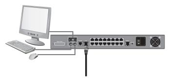
**2.4** Attach the power cord to the IEC power jack on the back of the Switch, and power up the Switch. (Refer to diagram below.)
